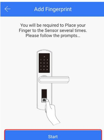
Scan your fingerprint on the lock four times.
