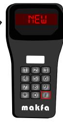
To transfer the handheld terminal's serial code to the safe, refer to the section "TRANSFER INFORMATION FROM THE HANDHELD TERMINAL TO THE SAFE". If the serial code of the handheld terminal differs from that of the safe, your handheld terminal will not function.
