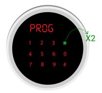
■ Input "842627", then press "#", "OLD" display input the master code (the factory set is "000000"), then press "#", "NEW" display.
