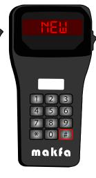
To transfer the handheld terminal's serial code to the safe, refer to the section "TRANSFER INFORMATION FROM THE HANDHELD TERMINAL TO THE SAFE". If the serial code of the handheld terminal differs from that of the safe, your handheld terminal will not function.
