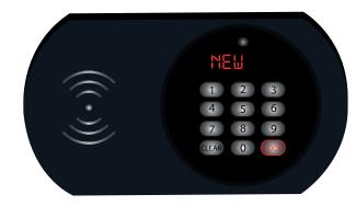
input 6 new master code, then press "Lock", "AGAIN"display, input again then press "Lock", "GOOD" display, show it is successful.
