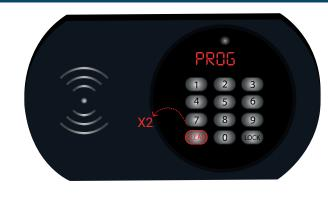
input "842627",then press "Lock", "OLD" display input the master code (the factory set is "000000"), tthen press "Lock", "NEW"display.
