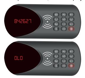
input 6 new master code, then press "Lock", "AGAIN"display, input again then press "Lock", "GOOD" display, show it is successful.
