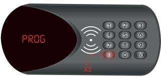
■ input "842627", then press "Lock", "OLD" display input the master code (the factory set is "000000"), tthen press "Lock", "NEW" display.
